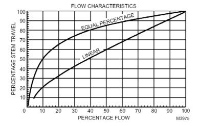
Fig. 2. Equal percentage and linear flow characteristics.
